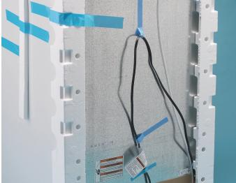
Secure movable components, tie down cords and temporarily attach surface and edge protection.
